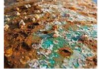
*Corrosion by chlorides:* On the surface of a stainless steel, pitting appears when the protective passive layer is broken in small isolated points and chlorides are deposited on the surface. The stainless steel, AISI304, supports well the chloride concentrations and other chemical levels recommended in swimming pool water. The material, AISI316, resists corrosion more than AISI304 not in a general way, but especially in the case of pitting corrosion.
