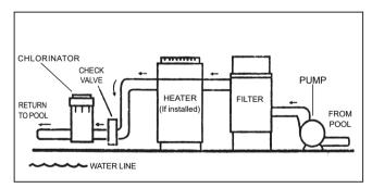
NOTE: Never install chlorine feeder directly into copper plumbing as pipe damage may occur. If you have brass or bronze backwash valves. or other sensitive metallic components. consult your dealer for precautions or recommendation for your particular system
