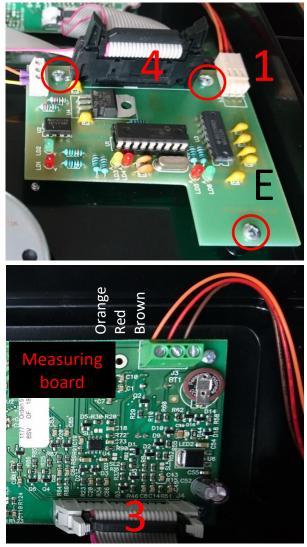
6. Connect the purchased RS485 VArio connection cables as follows (always respect polarity):
